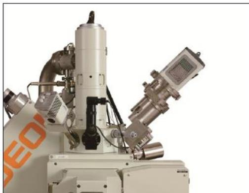
The SXES soft X-ray WDS Spectrometer mounted on a JEOL JXA-8230 EPMA.
